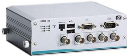
The **tBOX100-838-FL** transportation controller is based on a low power quad-core Intel Atom® processor (the E3845), and it comes with up to 4 Gbytes of onboard DDR3L memory. It features five BNC connectors for one audio-in and four video-in data streams. This fanless transportation computer is also accompanied by a capture SDK to allow system developers to speed up the embedded system development for transportation applications.
