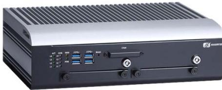
The **tBOX324-894-FL** is also equipped with two DDR4-1866/2133 SO-DIMM slots for up to 32 Gbytes of system memory. It offers a modular I/O design for integration into a variety of transportation applications. That includes security surveillance, transportation controller, truck fleet management, train management and onboard infotainment controller in vehicle, railway and marine designs.
